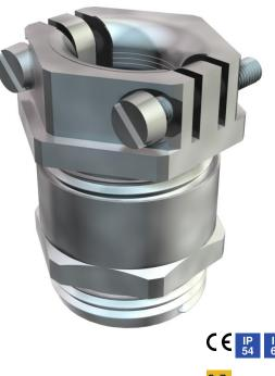
Cable gland with centrically acting transverse clip strain relief in the pressure screw, bend protection of movable cables through strongly rounded pressure screw.
