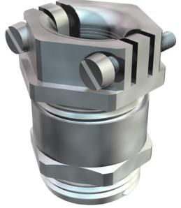
Cable gland with centrically acting transverse clip strain relief in the pressure screw, bend protection of movable cables through strongly rounded pressure
