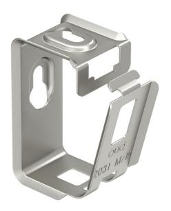
Metal grouped support for high mechanical stability, even in case of fire. Suitable for safe mounting above fire protection ceilings. Also approved as a cable-specific variant for the maintenance of electrical function to DIN 4102 Part 12. For wall and ceiling mounting. Lock can be opened without tools. Detailed information on the approved routing variants can be found in the appropriate testing documenta-
