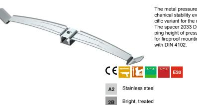
The metal pressure clip is halogen and fire load-free, and maintains a good mechanical stability even in fires. The pressure clip is also approved as a cable-specific variant for the maintenance of electrical functionality to DIN 4102 Part 12. The spacer 2033 D 15 x 3 G (must be ordered separately) increases the clamping height of pressure clips from 10 to 13 mm. The pressure clips are suitable for fireproof mounting above suspended fire protection ceilings in accordance with DIN 4102.
