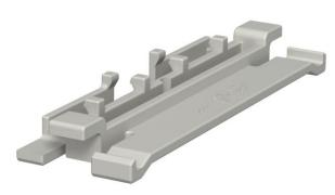
Cover clip for better and easier laying of lines in the WDK trunking. The cover fixing device can be moved along the entire length of the trunking. The cover clip is locked on one side and moved forward. This provides a 30° opening, meaning that cable routing is very simple. From trunking widths of 110 mm, the cover clips can also be used as a mounting
