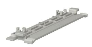
Cover clip for better and easier laying of lines in the WDK trunking. The cover fixing device can be moved along the entire length of the trunking. The cover clip is locked on one side and moved forward. This provides a 30° opening, meaning that cable routing is very simple.
