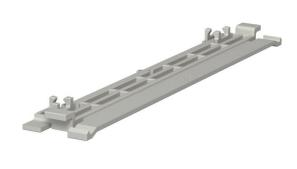
Cover clip for better and easier laying of lines in the WDK trunking. The cover fixing device can be moved along the entire length of the trunking. The cover clip is locked on one side and moved forward. This provides a 30° opening, meaning that cable routing is very simple.
