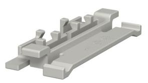
Cover clip for better and easier laying of lines in the WDK trunking. The cover fixing device can be moved along the entire length of the trunking. The cover clip is locked on one side and moved forward. This provides a  $30^\circ$  opening, meaning that cable routing is very simple.
