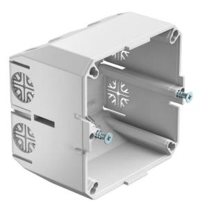
Accessory mounting box for the installation of devices with support rings and support clamps in WDK cable routing trunking of 60 mm trunking height. The device socket is placed on the floor connectors and fastened in the centre with a holt
