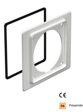
Adapter flange for mounting CEE 16 A sockets. During the mounting of the CEE mounting box, the adapter flange is mounted behind the trunking cover for accessory mounting boxes. Suitable for 400 V CEE 16 A 5-pin 6h, art. no. 6109874.
