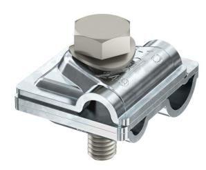
Quick connector to create T, cross and parallel connections. Mounting with stainless steel M10 x 40 screws. Suitable for reinforced steels  $\emptyset$  6–16 mm and flat conductors  $\emptyset$  8–10 mm. Conforms to the requirements according to DIN VDE 0185-305 (IEC 62305).
