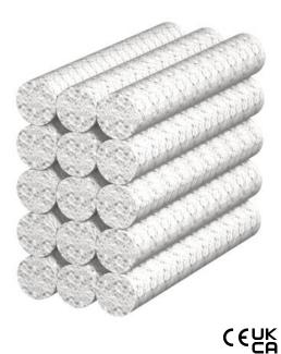
The noise limit barrier is used to reduce the transmission of airborne noise, e.g. when the trunking system is run through a wall between two offices. The noise limit barrier is made of glass wool, which, when delivered, has a diameter of approx. 30 mm and a length of approx. 300 mm. The material need not be greatly compressed during mounting.
