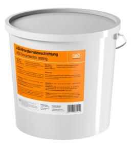
Combined, endothermic and weatherproof coating for internal and external areas. Universal protection coating for cable and cable support structures. Use as direct filler, and as paint when stirred. Sufficient for an area of 4 m<sup>2</sup>. Material class DIN 4102 - B2, normally flammable.
