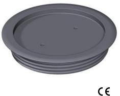
Blind cover for flushfloor closure of an underfloor outlet US80 or an underfloor outlet box UDL2-80. Only suitable for dry-cleaned floors for indoor use. Cover with 5 mm floor covering recess.
