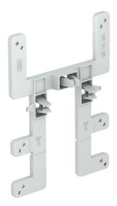
The fastening element BE TS GR can be used to attach OBO junction boxes, type T60 and T100, to mesh cable trays quickly and in a few actions. This keeps the junction box securely in position. However, it can be quickly dismantled as necessary.
