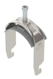
Clamp clip with U-foot, plastic pressure sleeve made of polypropylene. For vertical and horizontal mounting of 1 single cable on a C-profile rail. For slot width 18–22 mm. With 1-start screw thread on pressure sleeve, universal hexagonal screw head WAF10, with slot and cross recess. Suitable for assembly indoors and outdoors. We recommend the use of a counter-sleeve.
