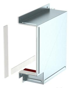
Fitting hood to cover two BSKM 1025 duct ends as flat angle for direct wall and ceiling mounting. Including glued-in seals for closing the joints and loose seals when combining with lock plate; screws for equipotential bonding also included.
