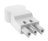
Socket section, 3-pin, type GST18i with screw connection for cables of 1.5–4.0  $\,$  mm² and for cable diameters between 10.5–14.5 mm (H05VV, NYM), unmounted with strain relief, terminable in situ, 250 V, 16 A.
