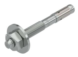
Bolt tie BZ3 for the anchoring of medium-duty to heavy-duty loads, both in cracked and non-cracked concrete. Suitable for heavy loads with small edge and axial distances. For knocking in.
