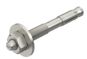
Bolt tie BZ for the anchoring of medium-duty to heavy-duty loads, indoors and outdoors, both in cracked and non-cracked concrete. It combines high approved loads with small edge distances and axial spacings.
