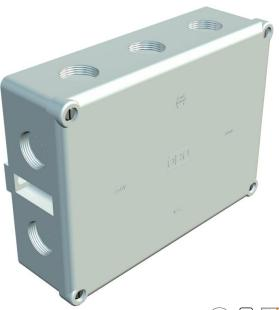
Protection rating IP54, nominal voltage 660 V, nominal cross-section  $16 \div mm^2$ , two fastening holes for screws up to 6 mm Ø on the outside of the box. Four cover screws, 10 break-out entries with thread M25 x 1.5. Clear internal dimensions: 178x126x57 mm B 12 empty: without terminal strip
