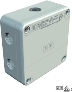
B9/T...: Comprises 2 halogen-free plastics components, 8 threaded entries (PG16) with push-through membrane (for cable diameter up to 15 mm)
