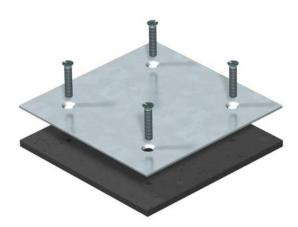
Lid blind plate for later blank covering of the DAT mounting opening. With rubber sealing plate for moisture protection according to DIN EN 50085-2-2, including fastening screws.
