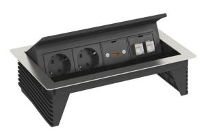
Foldable Deskbox with connection cable for fixed installation in a tabletop, housing made of brushed stainless steel with brush bar as cable outlet. Mounting is done via an installation opening 245 x 157 mm in the tabletop.
