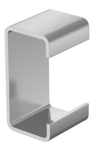
Spacer for use in US 5 supports. For static reasons, the spacer is always used to increase stability to prevent the support from deforming when the bracket is tightened with the hexagonal bolts.
