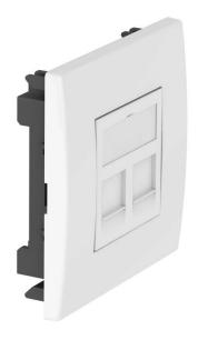
Installation unit to accommodate two type RM data technology modules, suitable for installation in Rapid 80 device installation trunking systems and ISS service poles. The type RM data technology support is suitable for accepting the following data connection modules: OBO (type): ASM-C5, ASM-C5 G, ASM-C6 and ASM-C6 G; R&M: Cat. 5 and Cat. 6 modules without support plate.
