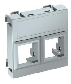
Data technology support with straight outlet and without a locking slider to accept two data technology connection modules with RJ45 socket. The locking fastening is suitable for horizontal and vertical installation in the system environment. Type LE has a special module seat and is designed for indirect fastening of the data connection modules in the mounting opening.
