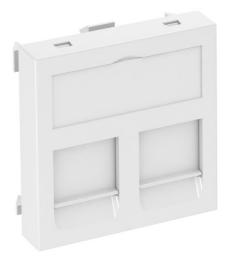
Data technology support with straight outlet and locking slider to accept two data technology connection modules with RJ45 socket. The locking fastening is suitable for horizontal and vertical installation in the system environment. Type B has a mounting opening of 19.35/21.55 x 14.85 mm and is designed for direct fastening of the data connection modules in the mounting opening.
