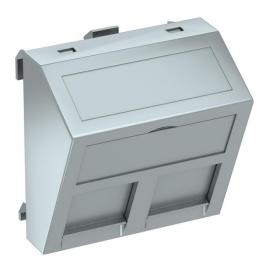
Data technology support with slanting outlet and locking slider to accept two data technology connection modules with RJ45 socket. The locking fastening is suitable for horizontal and vertical installation in the system environment. Type C has a mounting opening of  $19.30 \times 14.80 \, \text{mm}$  and is designed for direct fastening of the data connection modules in the mounting opening.
