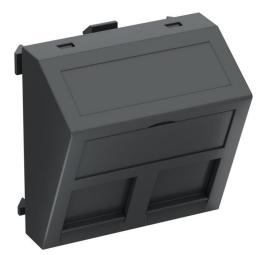
Data technology support with slanting outlet and locking slider to accept two data technology connection modules with RJ45 socket. The locking fastening is suitable for horizontal and vertical installation in the system environment. Type C has a mounting opening of  $19.30 \times 14.80$  mm and is designed for direct fastening of the data connection modules in the mounting opening.
