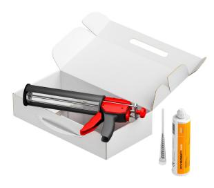
The PYROSIT® NG Starter Set contains all the required products to create foam insulations. The complete set consists of a PYROSIT® NG cartridge, two mixing tubes and a cartridge pistol. Suitable for 5:1 coaxial cartridges. For interior application.
