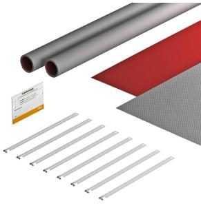
Complete set for covering cable bundles or cable support systems without cover to prevent a fire spreading. Application in outdoor areas. Each of the sets contains 4 sections of the weather-resistant cable bandage PYROWRAP® Wet, 8 metal strip clips and an identification plate. Sufficient for approx. 2 m length.
