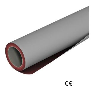
Weatherproof fire protection jacketing made of flexible mesh with fire protection coating to prevent fire spreading via cables and cable support systems. External side grey, internal side red. One roll contains 22 m<sup>2</sup>.
