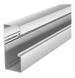
Device installation trunking Without base perforation suitable for direct wall mounting or mounting on panels. Over-lengths up to 6,000 mm for trunking bases and covers as well as other RAL colours can be provided on request. The visible surfaces of the device installation trunking are laminated. The cover must be ordered separately. We recommend the use of the duct clamp. Note:
