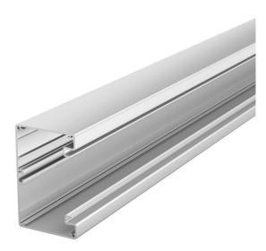
Device installation trunking Without base perforation suitable for direct wall mounting or mounting on panels. Over-lengths up to 6,000 mm for trunking bases and covers as well as other RAL colours can be provided on request. The visible surfaces of the device installation trunking are laminated. The cover must be ordered separately. We recommend the use of the duct
