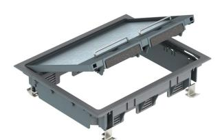
Service unit for 6 installation devices in 3 UT universal supports for use in raised floors for indoor use. Fastening bracket in a clamping range of up to 50 mm plate thickness.
