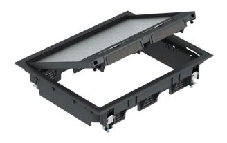
Separate fastening brackets must be ordered for raised floor mounting. Up to 6 installation devices with 50 mm central plate can be inserted. Service outlet with handle clamp, 3-compartment, for the installation of MT6 mounting support. Three type APMT2 cover plates can be installed.
