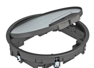
Service outlet with handle clamp for up to 10 individual Modul 45 devices in 2 UT3 and one UT4 universal support, use in duct systems and system floors for indoor use.
