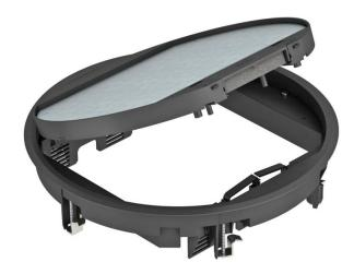
Service outlet with locking slider for up to 12 individual Modul 45 devices in 3 UT4 universal supports, use in duct and trunking systems and system floors.
