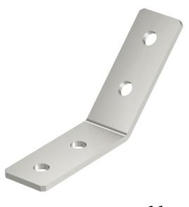
Mounting bracket with four holes to connect profile rails 41 x 41 mm and 41 x 21 mm at an angle of 45°.
