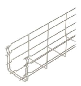
Mesh cable tray with shaped connector of side height 105 mm. No additional connection components are required for the mesh cable tray, it is simply interlocked. The grid width is 50 x 100 mm. Magnetic shield insulation without cover 15 dB, with cover 25 dB.
