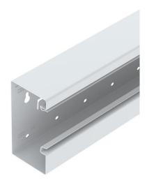
GS device installation trunking for mounting on the wall or on fastening panels. The GS device installation trunking possesses self-contacting locking straps to accept a sheet steel partition. The equipotential bonding between the trunking bases takes place using the trunking coupling. The protective measure and the equipotential bonding is guaranteed between the cover and the base by the self-contacting trunking cover. The real system opening is 76.5 mm. The cover must be ordered separately.
