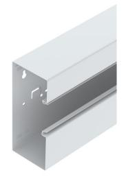
GS device installation trunking for mounting on the wall or on fastening panels. The GS device installation trunking possesses self-contacting locking straps to accept a sheet steel partition. The equipotential bonding between the trunking bases takes place using the trunking coupler. The protective measure and the equipotential bonding is guaranteed between the cover and the base by the self-contacting trunking cover. The real system opening is 76.5 mm. The cover must be ordered separately.
