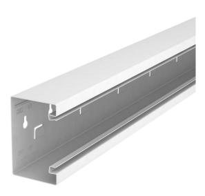
GS device installation trunking for mounting on the wall or on fastening panels. The GS device installation trunking possesses self-contacting locking straps to accept a sheet steel partition. The equipotential bonding between the trunking bases takes place using the trunking coupling. The protective measure and the equipotential bonding is guaranteed between the cover and the base by the self-contacting trunking cover. The real system opening is 76.5 mm. The cover must be ordered separately.
