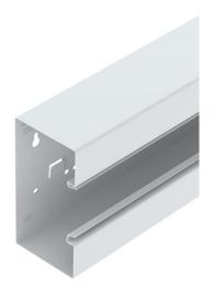
GS device installation trunking for mounting on the wall or on fastening panels. The GS device installation trunking possesses self-contacting locking straps to accept a sheet steel partition. The equipotential bonding between the trunking bases takes place using the trunking coupling. The protective measure and the equipotential bonding is guaranteed between the cover and the base by the self-contacting trunking cover. The real system opening is 76.5 mm. The cover must be ordered separately.
