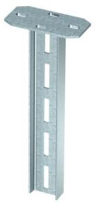
I support with welded head plate. For fastening to horizontal concrete ceilings and steel girders. Single and double-sided brackets of type AS 15, AS 30 and AS 55 can be fastened to the IS 8 K suspended support. The height of the brackets is infinitely adjustable.
