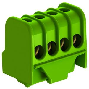
Protective conductor connection terminal strip, brass, steel screws, electrogalvanised and transparently passivated, nominal cross-section 6  $\div$  16  $\text{mm}^2\text{, nominal}$ voltage 400 V, 1-pole, with terminal sockets, max. connectable conductors per terminal 4 x 16 mm<sup>2</sup>, 4 x 10 mm<sup>2</sup>, 8 x 6 mm<sup>2</sup> or 12 x 4 mm<sup>2</sup>.
