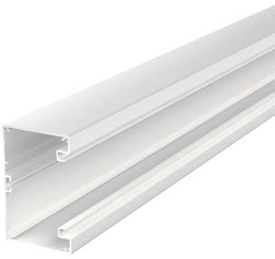
Device installation trunking without base perforation for direct wall mounting or mounting on panels. Over-lengths up to 6,000 mm for trunking bases and covers as well as other RAL colours can be provided on request. The visible surfaces of the painted device installation trunking are laminated.
