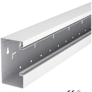
GS device installation trunking for mounting on the wall or on fastening panels. The GS device installation trunking possesses self-contacting locking straps to accept a sheet steel partition. The equipotential bonding between the trunking bases takes place using the trunking coupling. The protective measure and the equipotential bonding is guaranteed between the cover and the base by the self-contacting trunking cover. The real system opening is 76.5 mm. The cover must be ordered separately.
