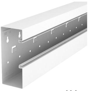
GS device installation trunking for mounting on the wall or on fastening panels. The GS device installation trunking possesses self-contacting locking straps to accept a sheet steel partition. The equipotential bonding between the trunking bases takes place using the trunking coupling. The protective measure and the equipotential bonding is guaranteed between the cover and the base by the self-contacting trunking cover. The real system opening is 76.5 mm. The cover must be ordered separately.
